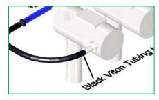
**Secure and route all tubing connections.** Take care to ensure the high temp. tubing is routed away from and will not chafe/rub the hot mufflers. Secure all tubing connections with a small zip tie. Hint:
